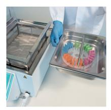
Transfer the now clean rack to tissue processor. Skip processor fixation step and process specimens in a shorter time.
