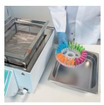
4 Place rack in transfer tray. For safe handling a cover is placed on the tray.
